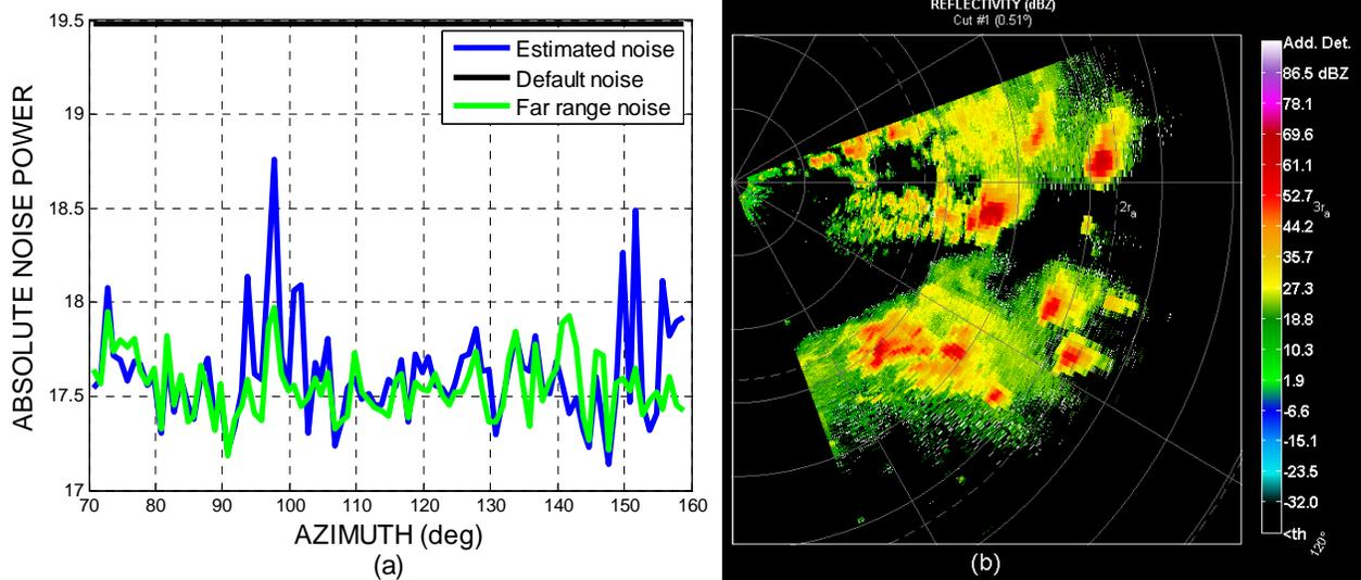
Fig. 4 (a) Noise estimates compared to the default and the far range noise, and (b) reflectivity field with additional detections obtained using estimated noise highlighted in white.
