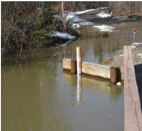
A new flood staff gage on Pile-driver Slough in Salcha helped emergency personnel and NWS forecasters respond to the 2009 spring breakup flooding.
