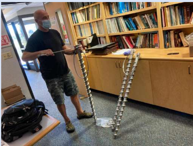
Mike Shanahan with the anchors and wrench used with the new antenna. Photo by Rick Hallman
