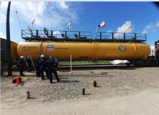
Tank Car designed to carry compressed or liquid commodities, like chemicals, molasses, edible tallow, water, and diesel fuel. Multiple types of fittings can be seen on the top which are used for demonstration purposes. Photo by Brian Miller
