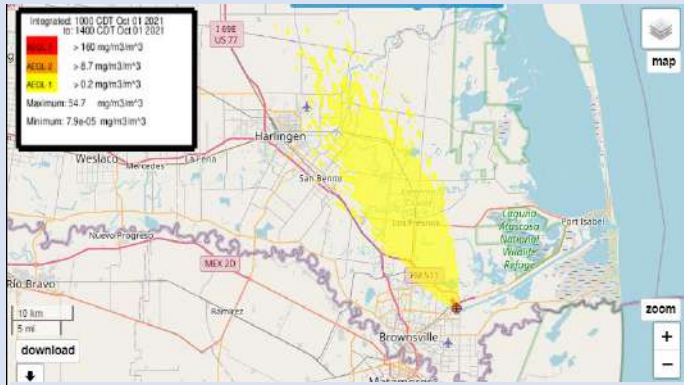
Above: Image A (left) - HSPPLIT model output showing a six hour leak of sulfur trioxide with light to moderate southeasterly winds. Image B (right) - Image A, at incident site.
