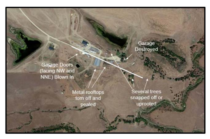
There was considerable damage to buildings on a local ranch. A shop building had 2 doors blown in and roof damage. Two other sheds had significant roof damage. Several metal rooftops were torn off and peeled back. A small garage was destroyed with a vehicle displaced inside, turned and moved by a couple feet. Several trees were snapped (approximately 1 foot diameter), with other smaller trees blown over or uprooted.
