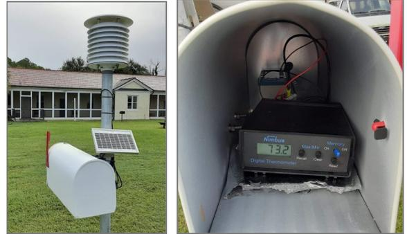
*This site on runs off of solar energy that charges a battery and connects to the temperature readout. The solar panel method is more energy efficient and allows for more accurate readings each day. The temperature display is called a NIMBUS and can save up to a month worth of daily observations.*
