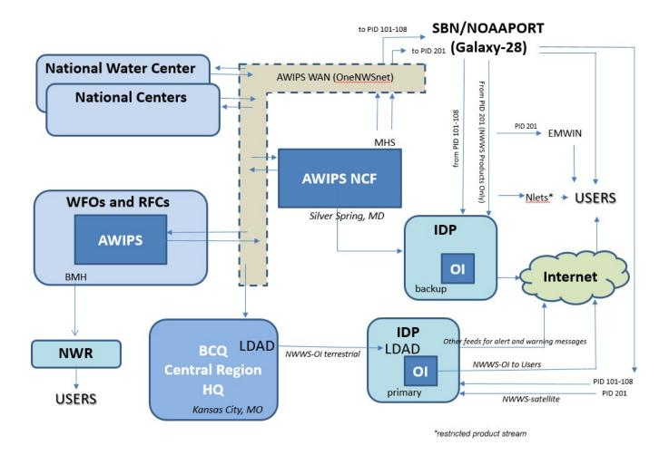
Figure 2.1 E-NWWS Enterprise Architecture Diagram; product flow
