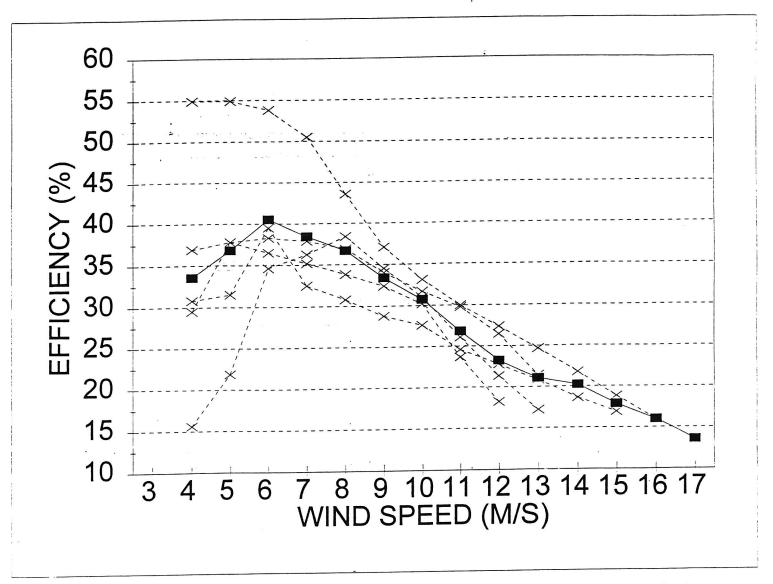
Figure 1. Overall efficiencies of 5 commercially available wind turbines in converting available wind power into electrical energy. The curve denoted by the dark boxes represents the average overall wind turbine efficiency.
