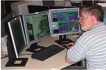
New AWIPS workstations provide vivid, flat-screen monitors (including an additional screen), more workspace, and vastly improved speed over its predecessor.
