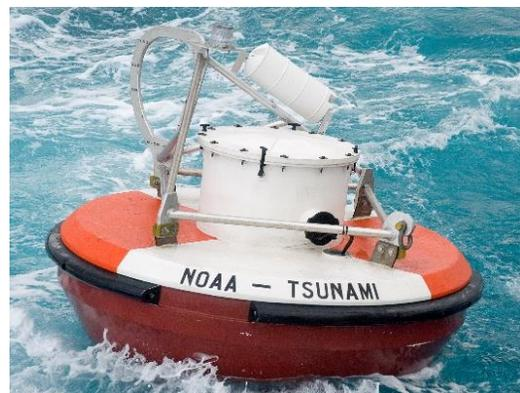
Figure 7. DART system buoy
