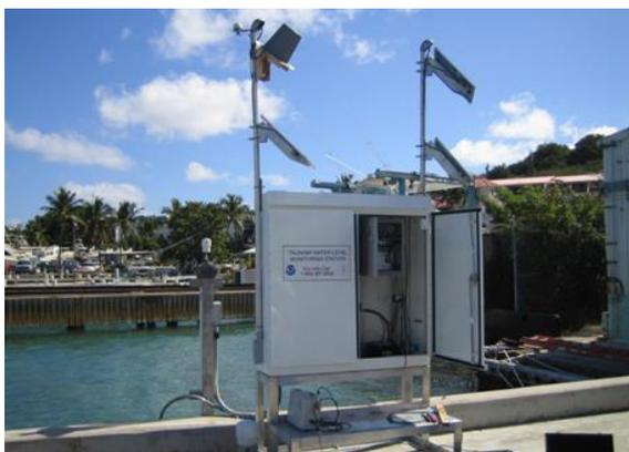
*Figure 8. Coastal water-level station*
