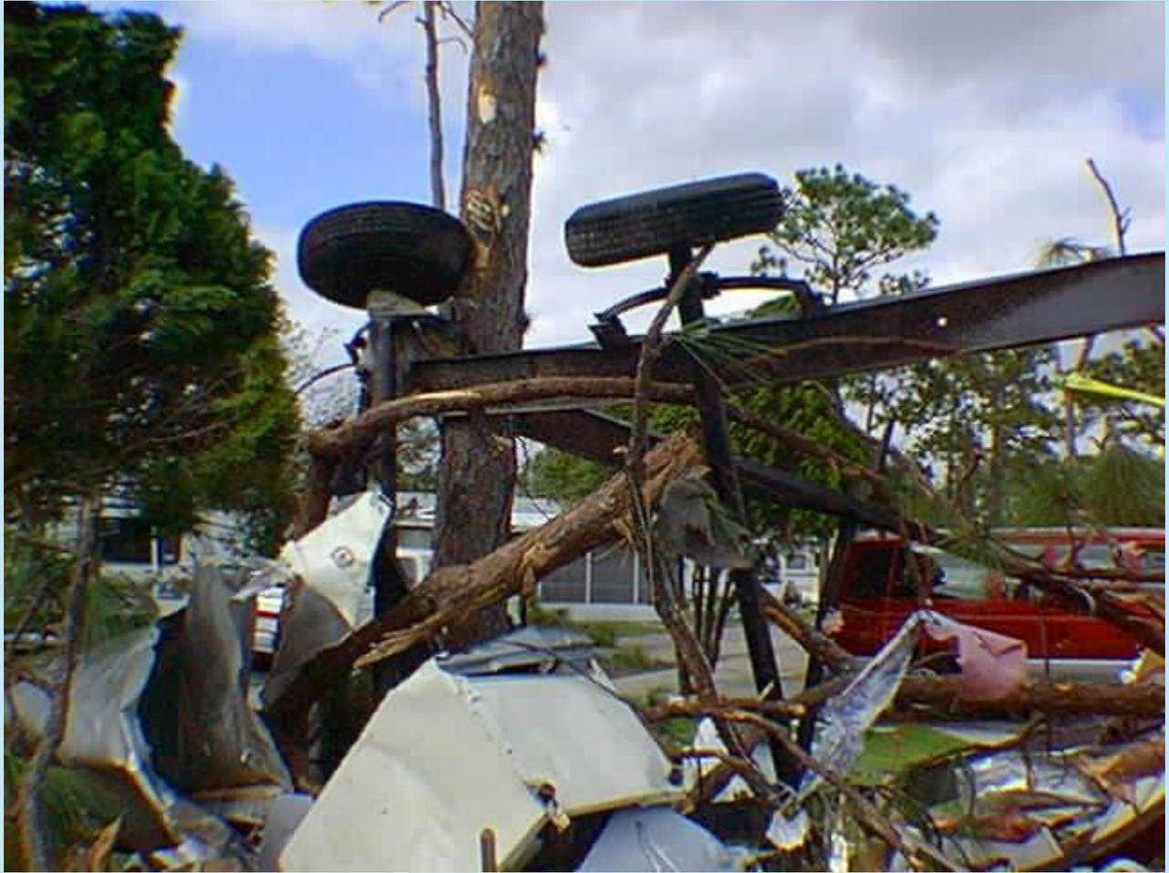
**RV frame wrapped around a tree. Note relatively undamaged areas nearby.**
