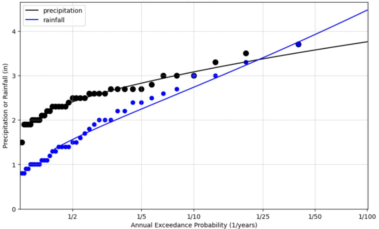
Figure 3: 24-hour precipitation (black) versus rainfall (blue) annual maxima, with GEV distributions fitted. Station is SNOTEL Site number 411 - Cool Creek at 1,914 meters. Precipitation and rainfall show differences at frequent AEPs, but converge at rarer AEPs.
