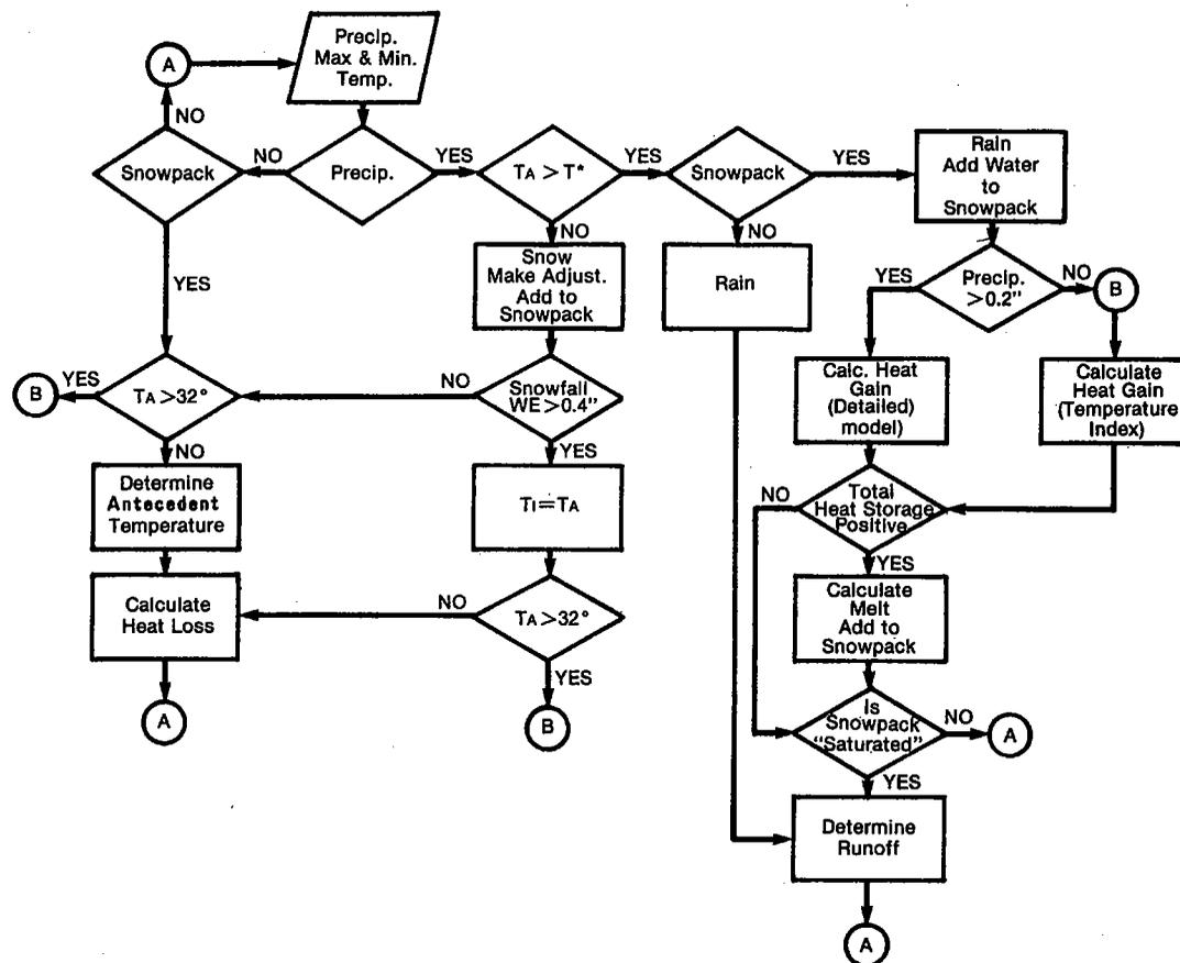
Figure 5.—Flow diagram showing principal features of the present adaptation of the NWSRFS snow accumulation and ablation model.
