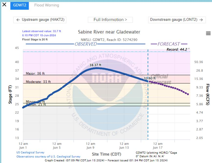
Figure 3. Example of a dynamic hydrograph.
