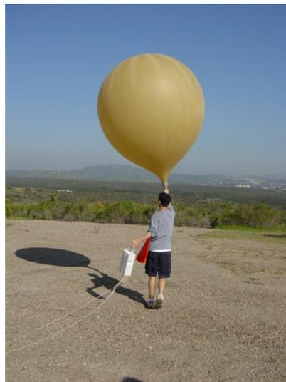
The typical weather balloon is about six feet in diameter (two meters) and is filled with either helium or hydrogen. It carries a one-pound (half
