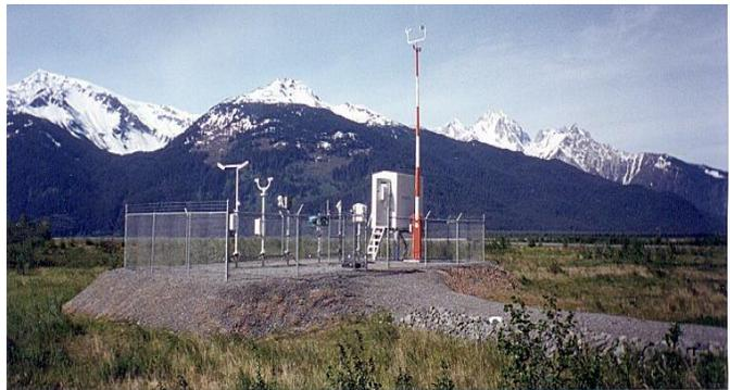
A network of **ALERT** (Automated Local Evaluation in Real Time) equipment is used primarily for hydrological purposes, measuring rainfall and river levels, but also temperature and wind in some cases. This equipment is maintained by flood control agencies in cooperation with the NWS.
