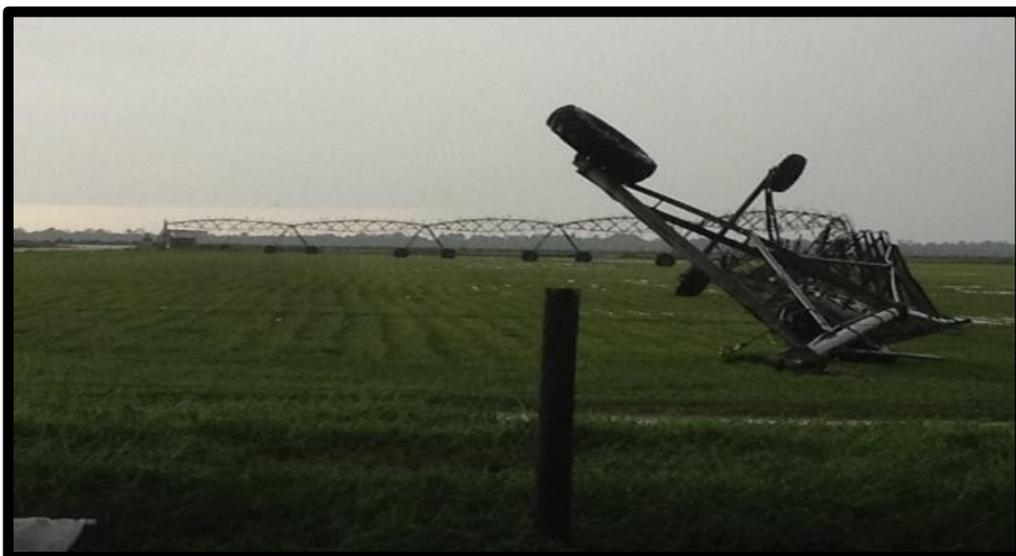
This photograph shows damage to a center point irrigation system at the sod farm which was toppled by winds estimated up to 75 MPH.
