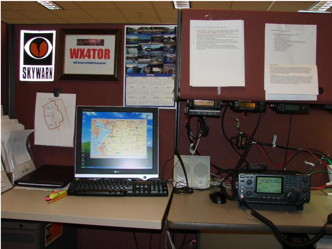
**WX4TOR is equipped with HF, VHF, and UHF radios for short and long range communication. Operating modes such as voice, packet, and APRS are used to collect real-time spotter reports and weather observations.**
