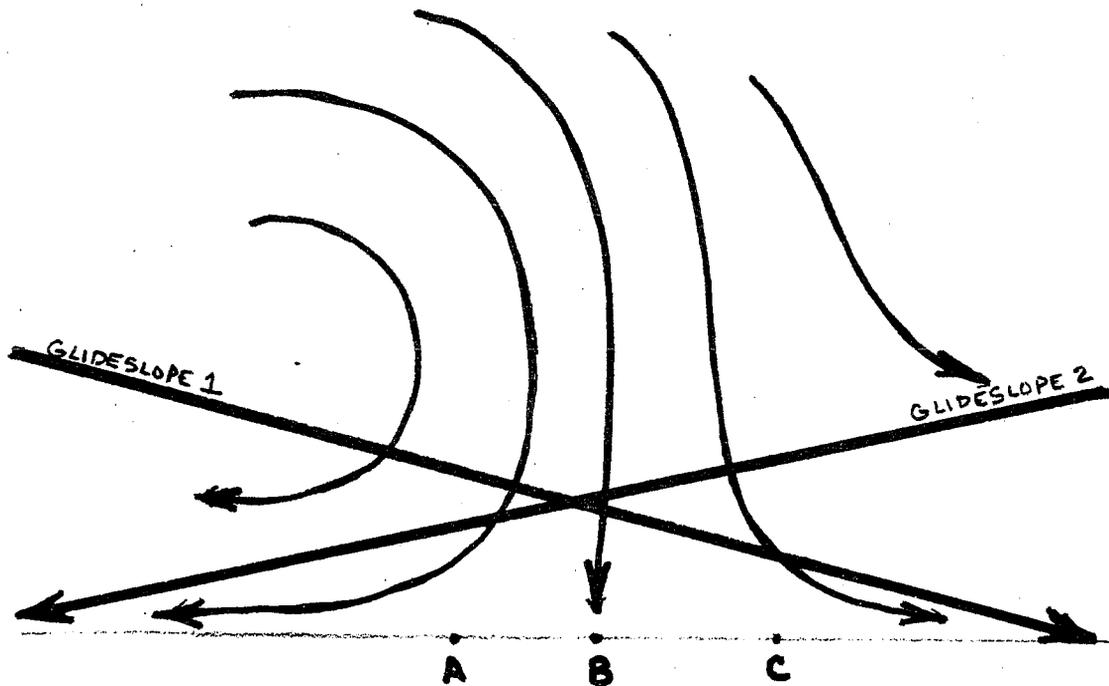
Figure 8. Vertical cross-section through axis of rotation of downdraft portion of rotory motion associated with strong windflow over a mountain barrier.
