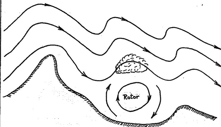
Figure 6. Rotor shear. Rotory action beneath terrain induced waves can produce shear and strong up and downdrafts over the valley.
