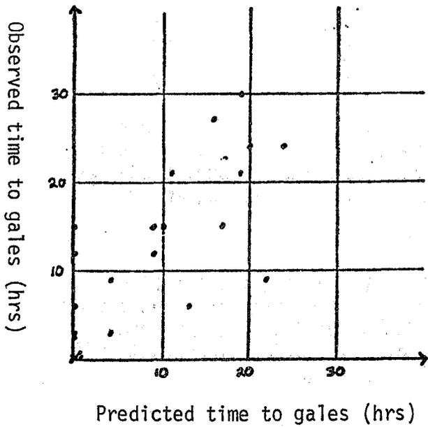
Figure 2. Predicted versus observed time to gale onset using Group 2 (1980-81) regression coefficients. Astoria to buoy 46005 pressure difference was 9-mb or greater and gales were subsequently observed. Data were for Winter 1980-81 only.
