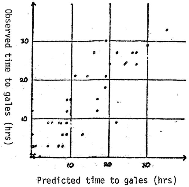
Figure 3. Predicted versus observed time to gale onset using Group 2 (1979-80) regression coefficients. Astoria to buoy 46005 pressure difference was 9-mb or greater and gales were subsequently observed. Data were combined for 1979 through 1981.
