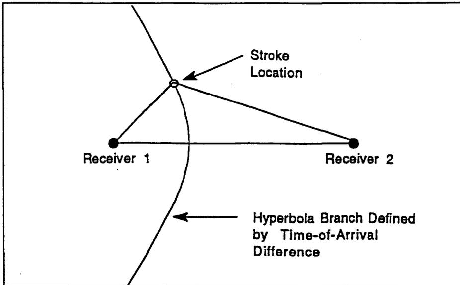
**Figure 3a:** Detection of a cloud-to-ground lightning stroke by two TOA receivers. For a given time-of-arrival difference, the stroke that emitted the signal could be located anywhere along one of the branches of a hyperbola that passes between the two receivers and has as foci the two receiver locations (from Holle and Lopez 1993).
