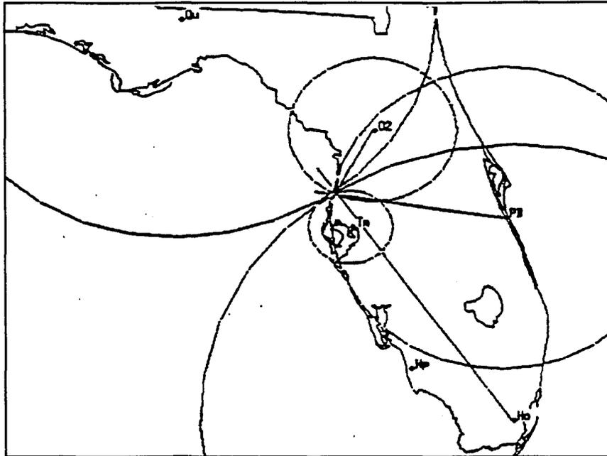
**Figure 4:** Example of a lightning stroke located by two LPATS sensors and three IMPACT sensors. Straight lines are azimuth vectors (i.e., DF) and circles are the solution radii (i.e., TOA). Figure from Cummins 1995.
