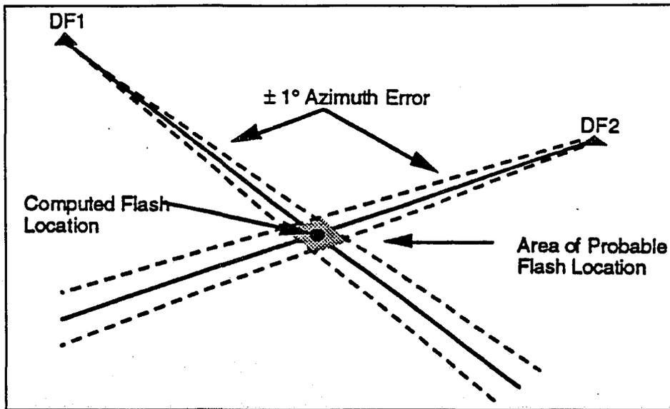
**Figure 2a:** Determination of cloud-to-ground flash location when two DFs detect it. Solid lines represent measured azimuth of the flash; dashed lines outline the angular random error in azimuth measurements. Dot indicates computed flash location; shaded indicates area where flash probably occurred (from Holle and Lopez 1993).
