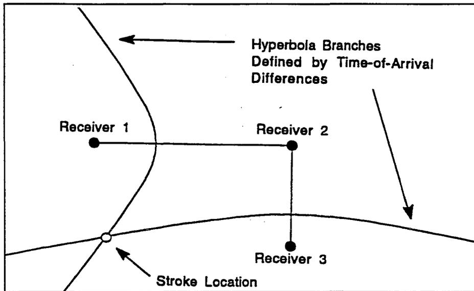
**Figure 3b:** Detection of a cloud-to-ground lightning stroke by three TOA receivers. Two non-redundant hyperbola branches are defined whose intersection can define the location of the stroke (open circle). From Holle and Lopez 1993.
