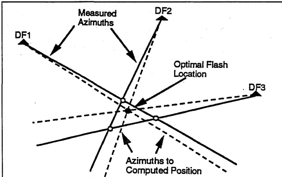
**Figure 2b:** Determination of flash location when three DFs detect it. Solid lines represent measured azimuths of flash. Open circles indicate the three possible locations defined by three different intersections of azimuth vectors. The position (solid dot) that would minimize the square differences between measured azimuths (solid lines) and computed azimuths (dashed lines). From Holle and Lopez 1993.
