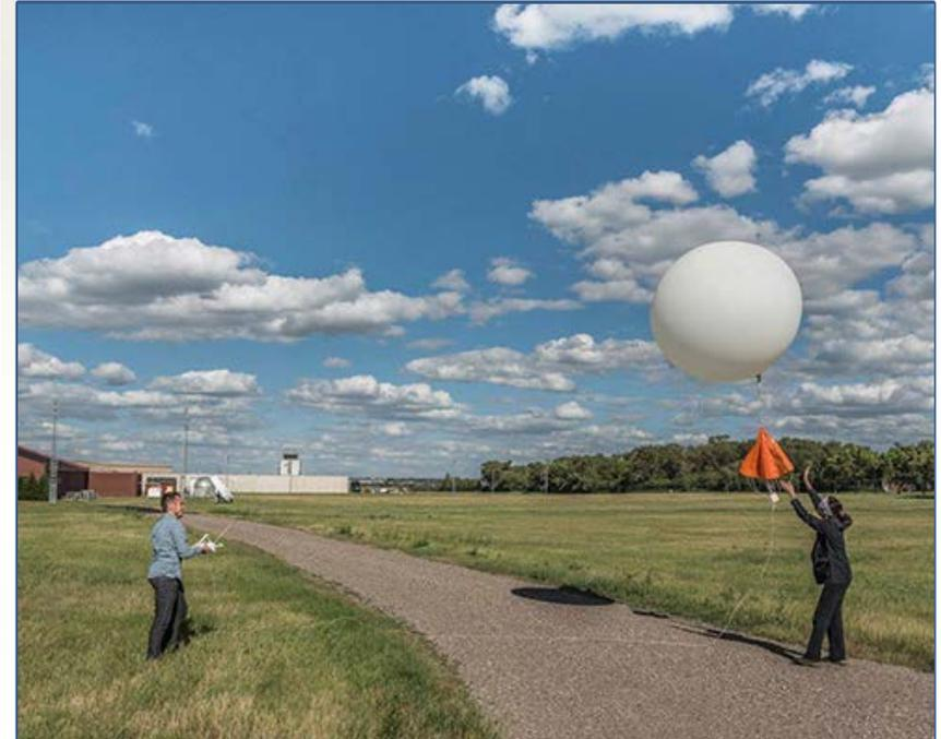
**Radiosonde Manual Launching Operation**
